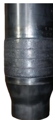
DRILL-GUARD Nb hardbanding deposit on a tool-joint
