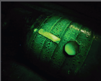
Wet mag particle testing performed on DRILL-GUARD Nb at Accu-Test labs in Houston, TX.
