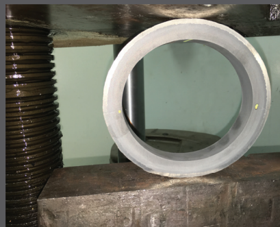
DRILL-GUARD sustained 26,647 lbs (12,086 kg) of force on a 1" (2.5 cm) Ring Test prior to yielding without any spalling, flaking, or delamination. The testing was performed at Accu-Test labs in Houston, TX.
