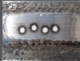
Every DRILL-GUARD batch has a six layer welded test and a spectrometer verifies that chemistry meets the stringent specifications.
