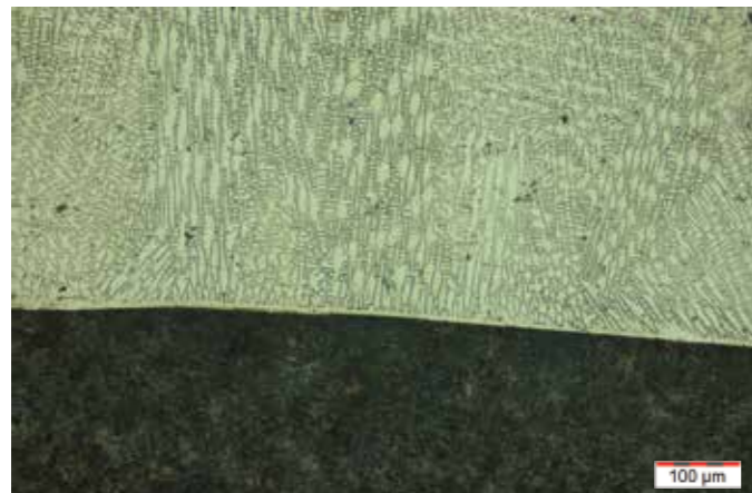
Micrograph showing the bonding between the base metal and the first layer
