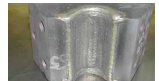
Forging die hardfaced with STELLOY 21-G
