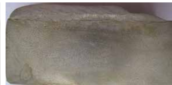
Cladding : First layer STELLOY 6-G Second layer STELLOY 6-G
