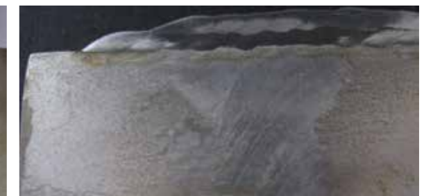
Cladding : First layer STELLOY 21-G Second layer STELLOY 6-G
