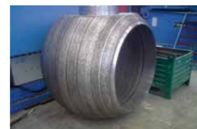
Ball valves hardfaced with STELLOY 21-G
