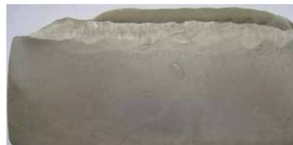
Cladding : First layer 309L Second layer STELLOY 6-G
