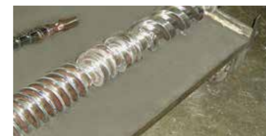
Extrusion screw hardfaced with STELLOY 12-G
