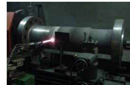
HVOF coating on turbine drive shaft
