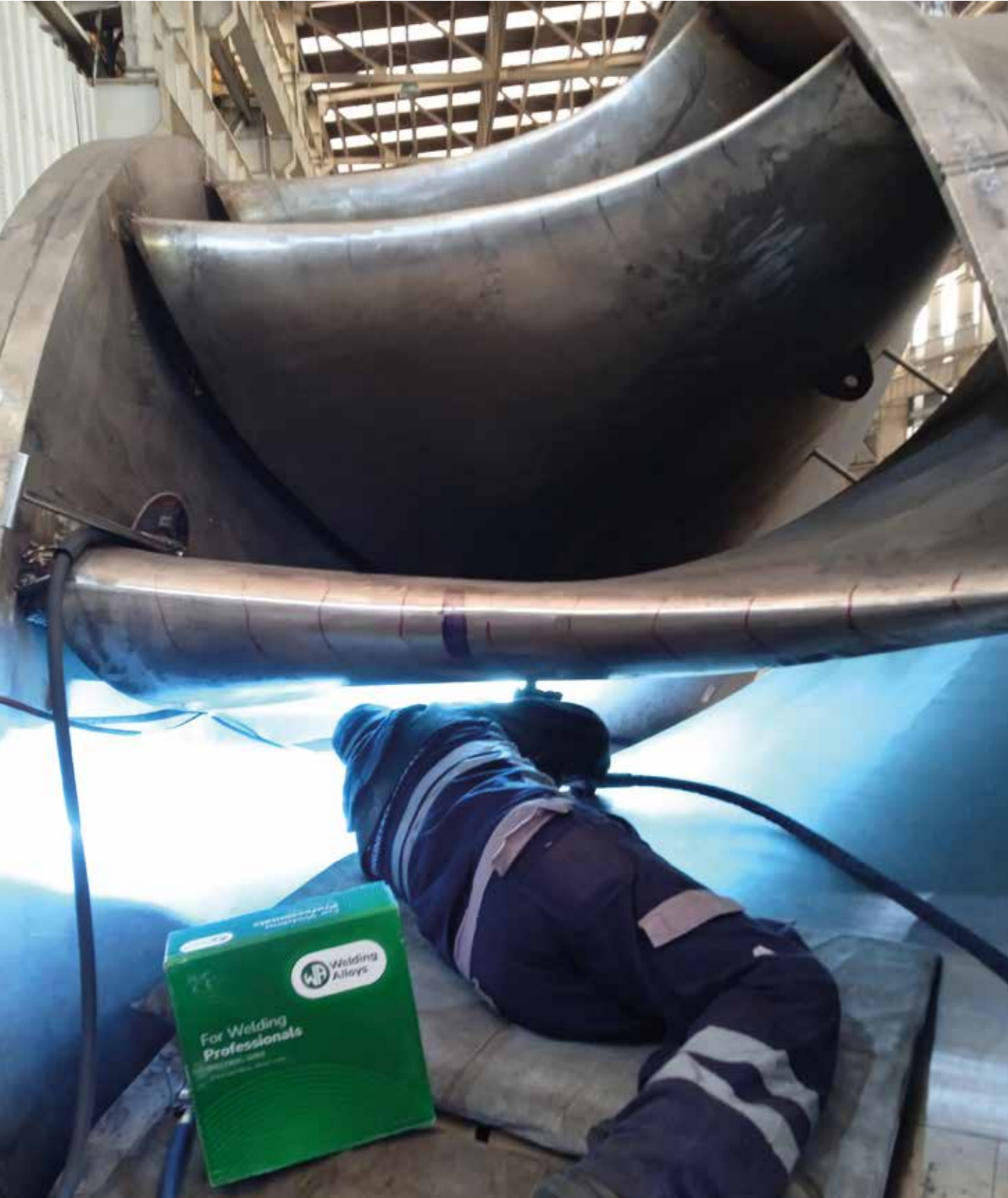
Francis turbine manufacturing using CHROME CORE M 410NiMo-G
