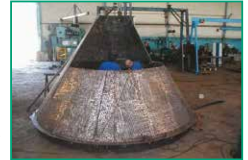
Classifier cone with double-sided Hardplate
