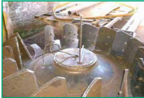
Fan blades protected with Hardplate or Hardlite
