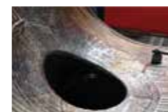
Restoration of cladding TETRA S 309L-G + 347L-G
