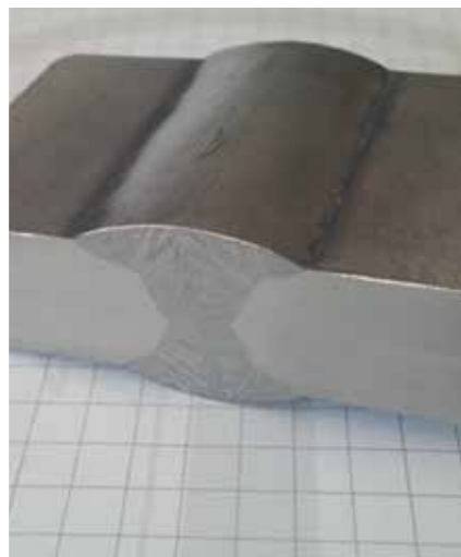
Two-run SAW 316L (Thk 15mm) TUBE S 316L-S
