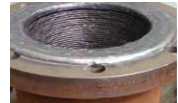
ID bore cladding in 347H TUBE S 743-G (one layer)
