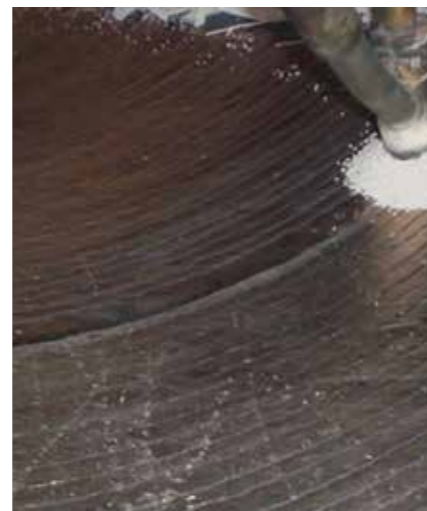
SAW cladding on 1.25%Cr-0.5%Mo TUBE S 309L-S + 308L-S
