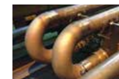
Furnace cracker TETRA V 309HT-G
