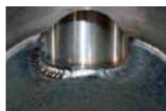
Small ID pipe cladding STELLOY 625-G (TIG)
